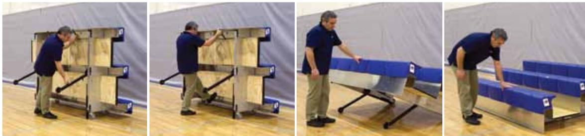
**One minute – one person.** We engineered MAXAM 1™ Portable Bleachers to be operated by a single person. Just extend each of the traction arms, tip the unit, give it a gentle push to lock it down, and it is ready to go. Gas struts provide a controlled descent and lift assistance to ensure easy operation. No more waiting for a crew or scheduling extra labor – just keep saving labor time and cost for the entire life of your seats.
